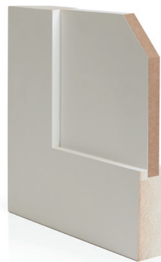
LAMINATED WOOD STILE AND RAIL CONSTRUCTION WITH MDF OVERLAY DOOR SKIN
